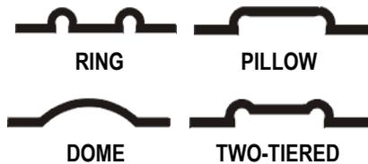
In the case of a ring emboss, borders are usually raised .005" to .010" high and .040" to .070" wide. The maximum emboss height is typically limited to 6 times material thickness of polyester and 9 times material thickness of polycarbonate. Embossed corners should have a minimum of .010" radii.
